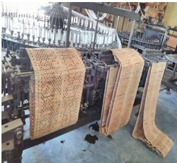
Figure 4. Lacemaking mechanism with punctured cards
