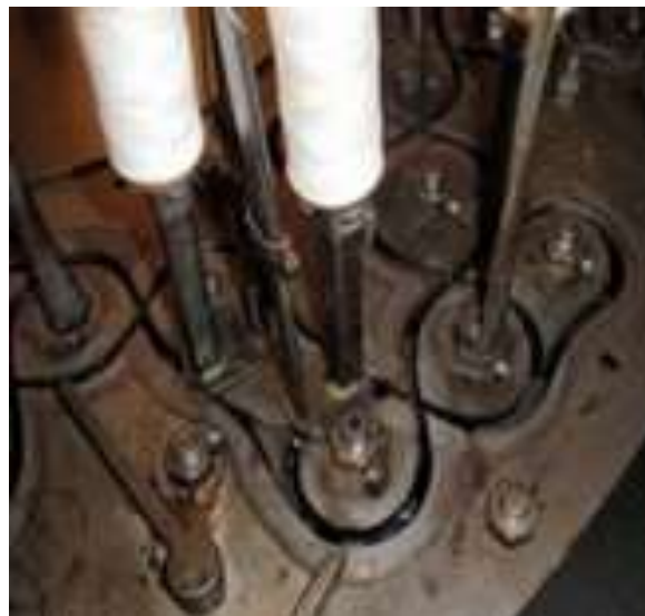
Figure 5. Mechanism detail—grooves and paths of bobbins with thread
