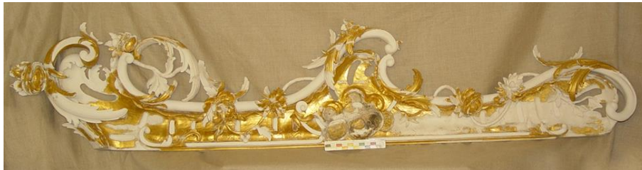
Figure 32. The right frame listel to the temple icon Nicholas the Wonderworker in Life in the process of preserving the historical levkas and local reconstruction of its losses, with the surface cleared of persistent contamination of historical gilding
